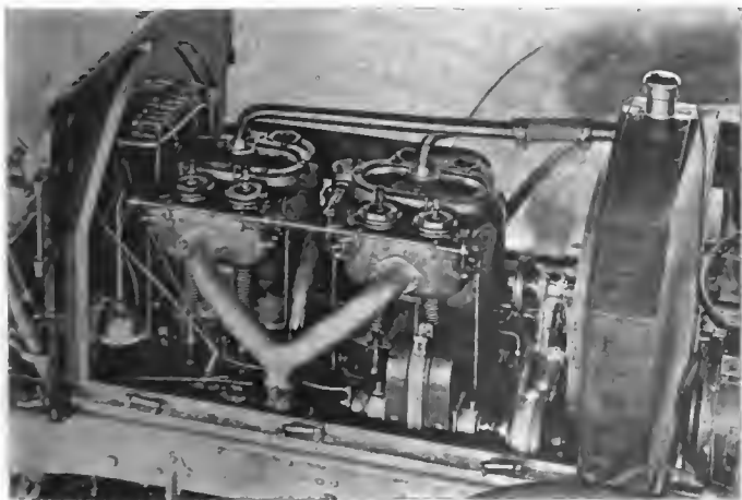
ADMISSION SIDE OF 40-HORSEPOWER LOCOMOBILE MOTOR.
